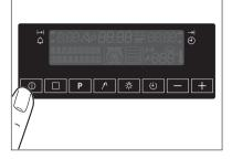
**2.** Press the main power ① and the clock function ④ buttons at the same time.
